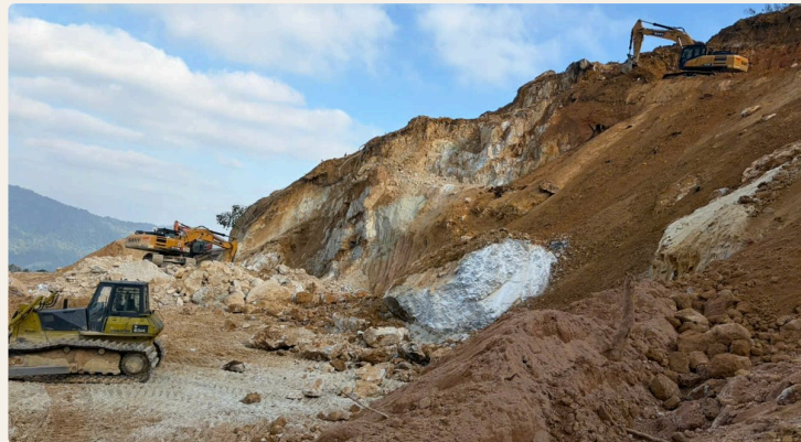
Selective blast + sort — FeSi-grade lump fraction
