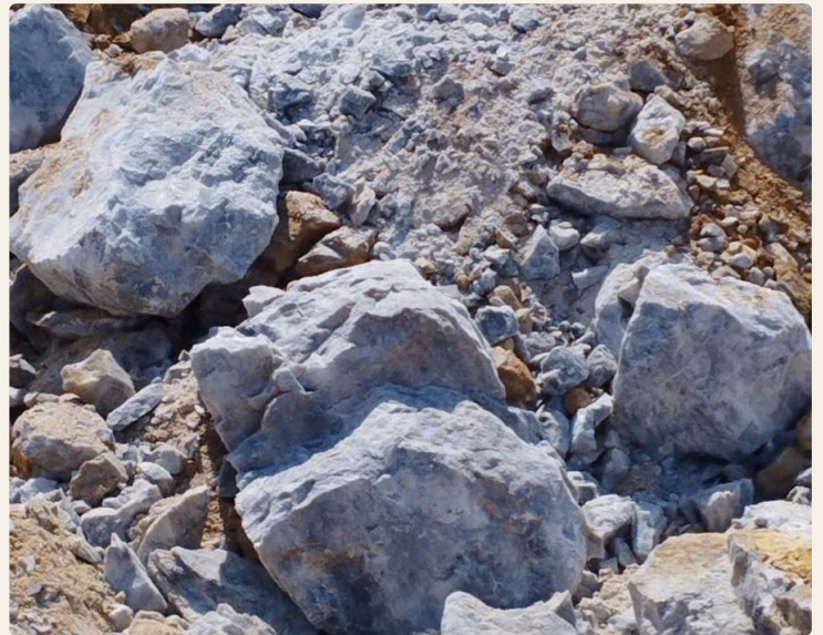
LLS lump quartz — 40–150 mm, FeSi-grade sizing
