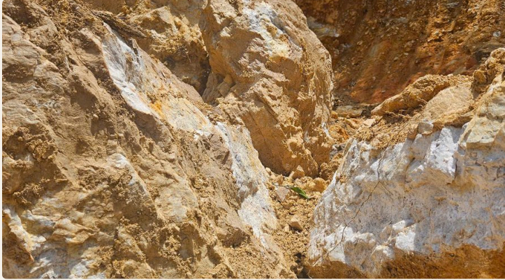
Vein quartz at pit face — high mechanical strength, low decrepitation
